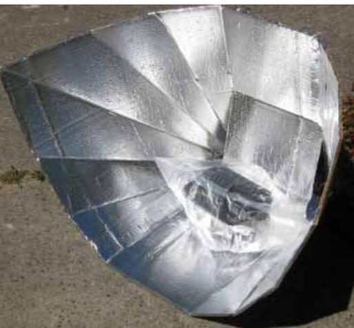
Solar cookers and ovens are by far the most energy-efficient cooking appliances. They reflect heat from sunlight to a central area to heat food or water.
